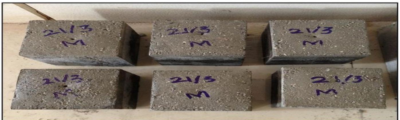
Fig-13 Processed geopolymer mortar cubes of 70x70x70mm
