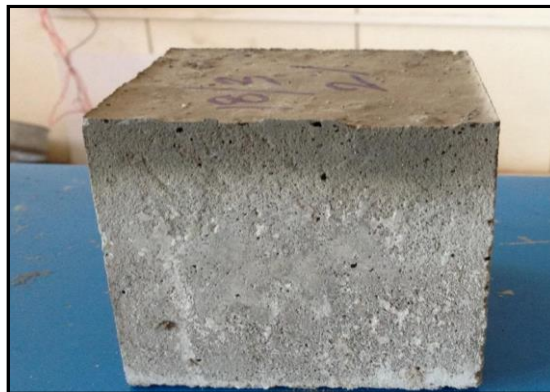
Fig-16 A distinct 12 to 15 mm thickness dark grey layer is observed from top of Rice husk ash replaced processed geopolymer concrete.
