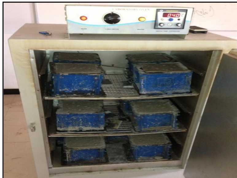
Fig-11 Oven Curing
