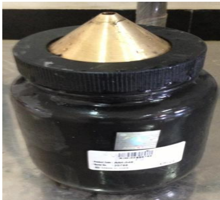
Fig-2 Pycnometer Bottle filled with Rice Husk Ash and Water.
