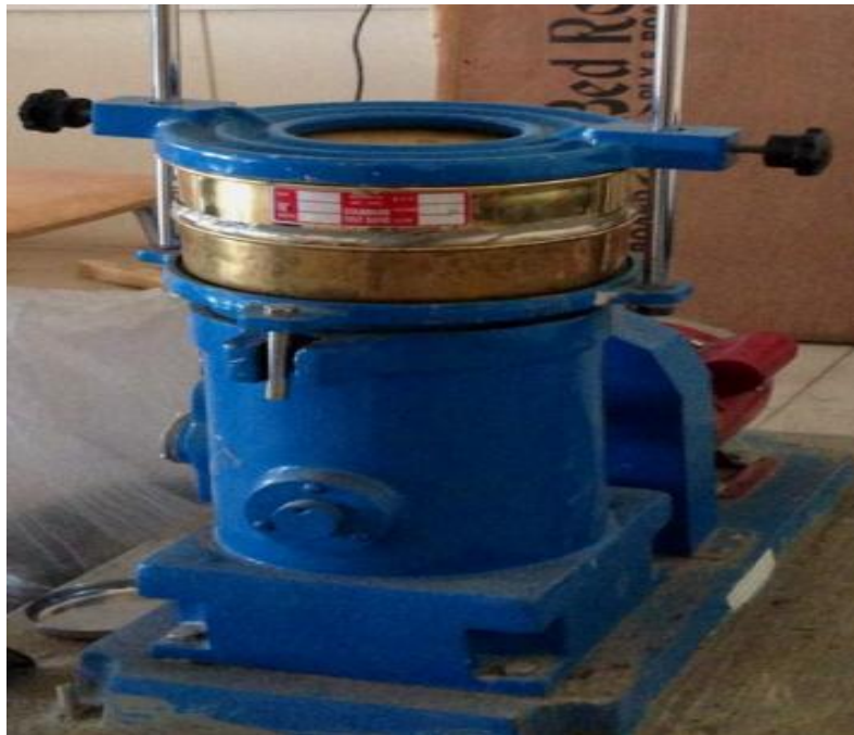
Fig-1 Mechanical Shaker with 45 \mu I.S. sieve with lid and receiver.
