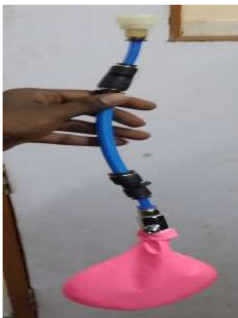
Fig -5: Gas collection set-up
