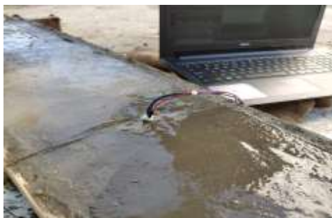
Figure – 6 Sensor embedded in beam
