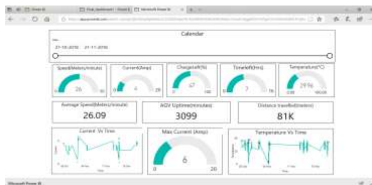
Fig-3: Main Dashboard (Current Values) of the system
