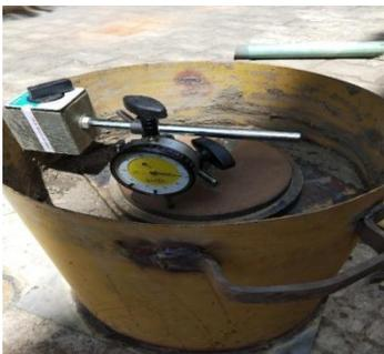
Here, to identify the behaviour of clay soil without stone column, the load is directly applied on the plate of 3.5kg, which is placed over the top of the clay soil. The settlement of clay soil is noted for every one minute and the graph is drawn between time and settlement for increase in load by 0.5kg.
