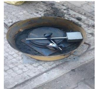
Here, to identify the behaviour of clay soil with encased stone column, firstly the clay soil is excavated using 6cm diameter pipe. Then the geogrid is placed in the hole and is filled with aggregates. Here we have taken square pattern arrangement of stone columns. Load is then applied on the plate. The settlement is noted for every one minute and the graph is drawn between time and settlement for increase in load by 0.5kg.
