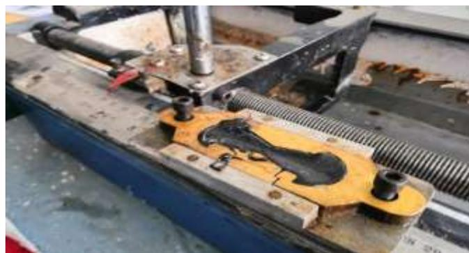
**Figure – 6: Ductility mould**
