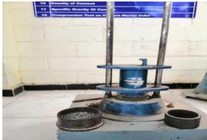
**Figure – 3:** Impact Testing Machine
