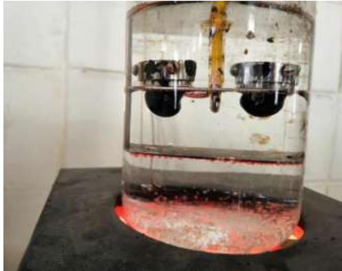
**Figure – 5: Ring and Ball Apparatus**
