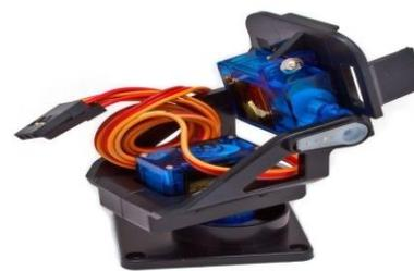
The pan and tilt servo rotates 180° from side to side and can tilt up and downward around 150°. This motor is a plain everyday analog servos we can use microcontroller or driver. The motor helps in fixing the camera when rotating and tilting it up and down.
