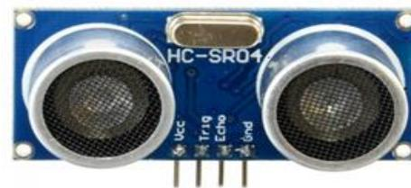
There are 4 pins in hc-sr04. Its operating voltage is +5volts. This is very popular sensor for measuring distance or for sensing objects. It has two eyes as shown in figure. The sensor works with the formula
