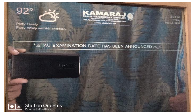
Fig – 7: Output – Weather, Institution Logo, Time & Date and Institutional Updates in Smart Mirror
