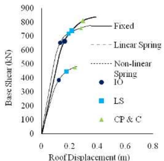
Fig. 6: Capacity curve in transverse direction
