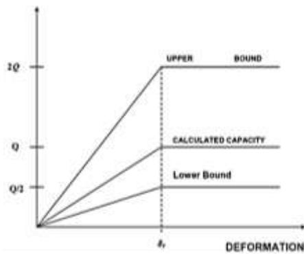
Fig. 4 : Idealized elasto plastic load-deformation behavior for soils (ASCE 41-17)
