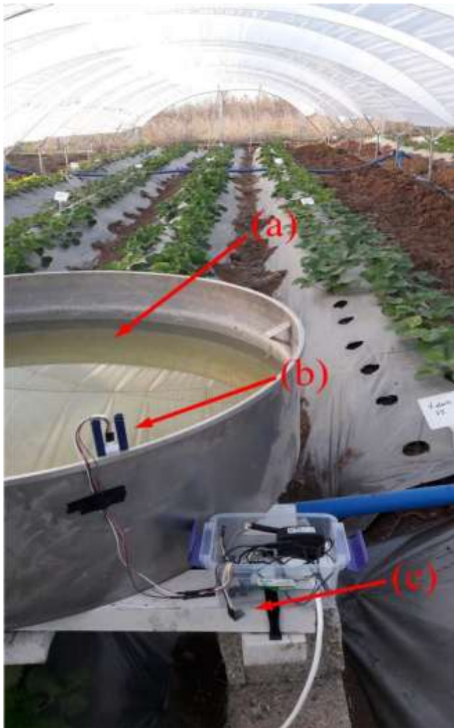
Fig. 3. Data gathering unit inside the greenhouse. (a) Evaporation pan, (b) Water level sensor, and (c) Environmental sensor. Most excellent quantity of water for pleasant crop exceptional truly makes contribution to modest water consumption on this planet.
