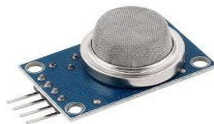
INTERFACING MQ2 WITH ARDUINO
