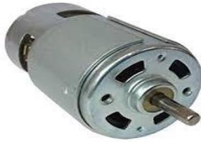
Here a dc servomotor (10 rpm) is used. They are also called as control motors. It works based on PWM (Pulse width modulation) principle, means its angle of rotation is controlled by the duration of applied pulse to its Control PIN. The required gears are connected to the motor through the help of a resistor for rotation of solar panel.
