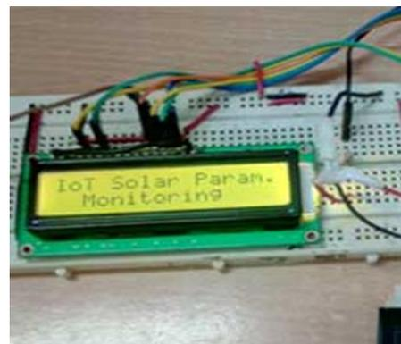
2) The solar panel parameters are also displayed and stored in an application or web page using the think speak IoT platform. So that the solar panel can be monitored remotely.
