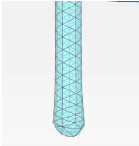
**Fig.6 Failed model GPA in PLAXIS 3D post loading**
