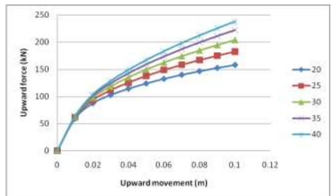
Fig 4. Uplifting force-Upward movement for L= 5m , D=0.5m for varied angle of internal friction of surrounding soils
