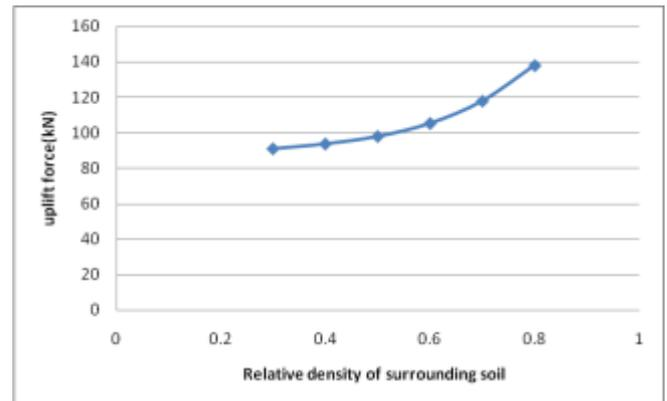
Fig. 3 Uplifting force- at movement of 10% Dia( 0.5m) and Span 5m for various relative densities..
