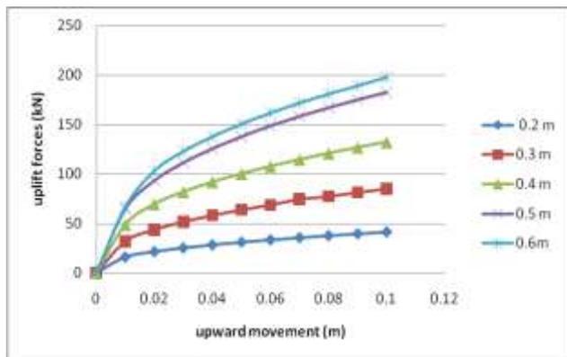
Fig 1 Uplifting force-upward movement plot for various Dias at Span of 5m
