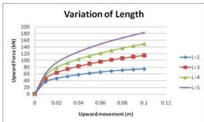
Fig -2: Uplifting force-upward movement plot for various spans with D=0.5m
