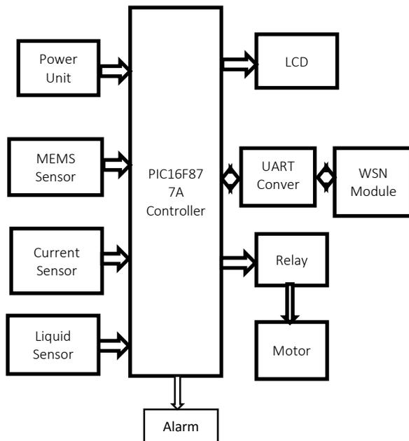
Figure: 1 Block Diagram of Motor Unit
