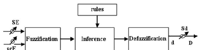
Fig - 9: Block diagram of fuzzy logic controller
