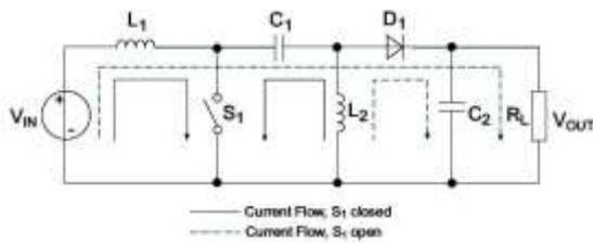
Fig - 2: Working of SEPIC Converter
