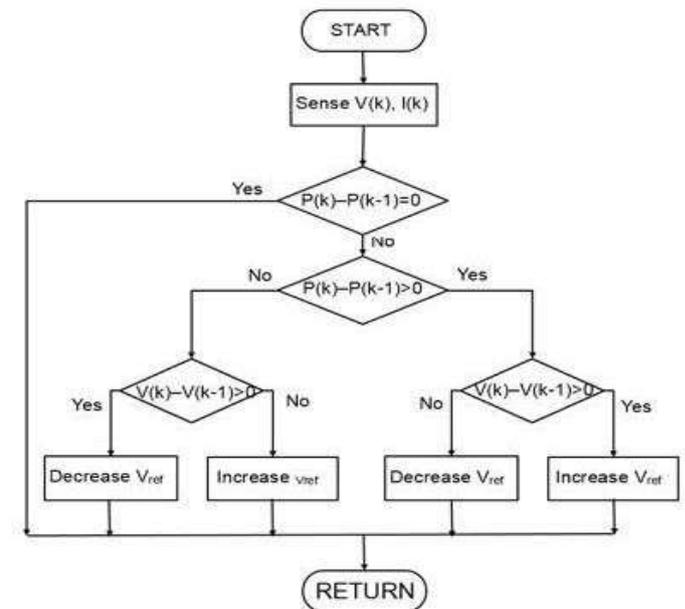
Fig - 8: Flowchart of Perturb and Observe algorithm
