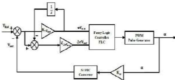
**Fig – 10:** Block diagram of fuzzy logic controller for SEPIC converter
