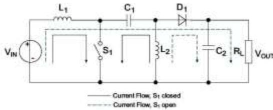
Fig - 2: Working of SEPIC Converter
