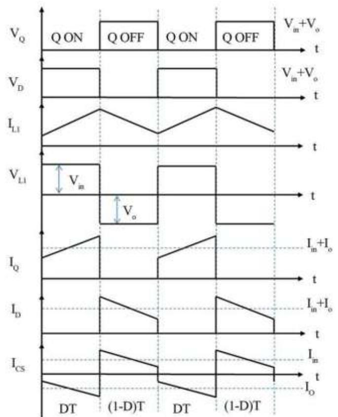
Fig - 4: Waveform of SEPIC Converter
