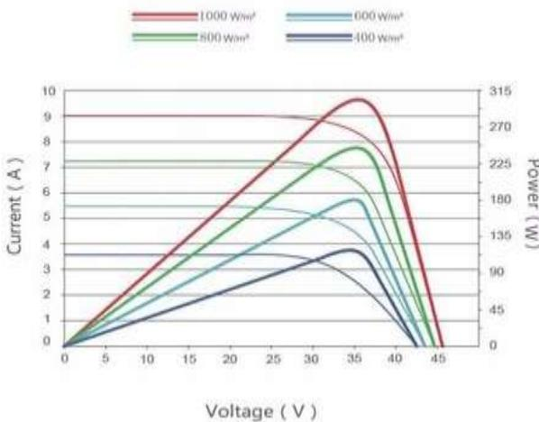
Fig - 5: General P-V Characteristics of PV panel
