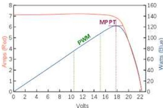
Fig - 6: P-V Characteristics of PV panel after implementing MPPT technique
