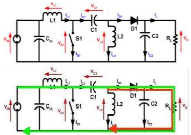
Fig - 3: Circuit Diagram when switch S1 is open
