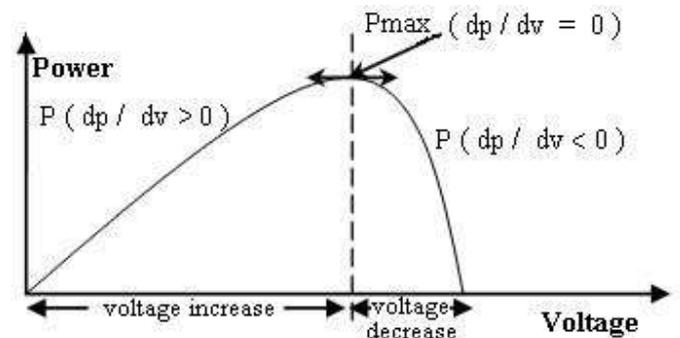
Fig - 7: P-V characteristics after employing MPPT Technique in SEPIC converter topology
