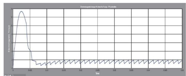
Fig. 8. Electromagnetic torque Vs time for Fuzzy – PI controller.
