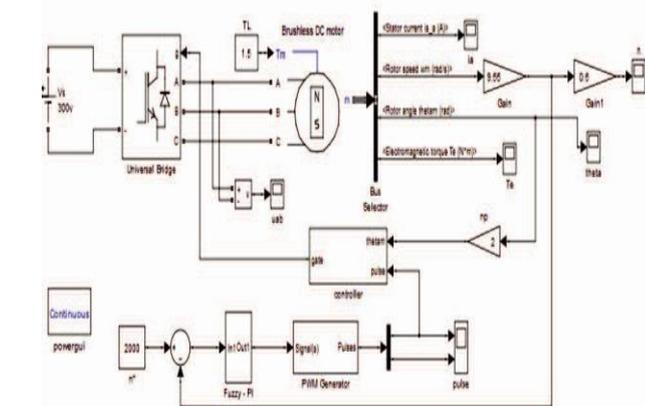
Fig. 4. Simulink model of BLDC motor using Fuzzy-PI controller
