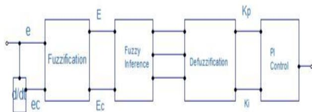
Fig. 3. Structure of Fuzzy tuned PI controller
