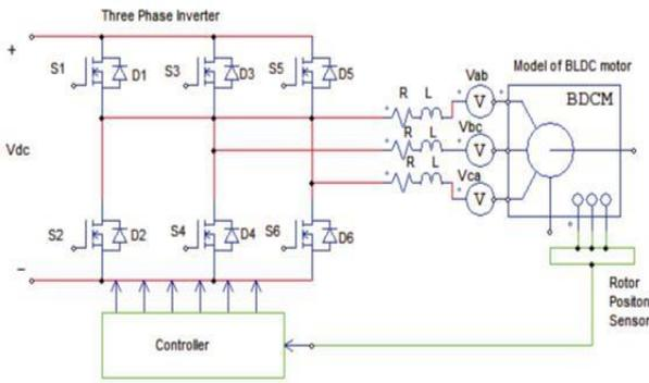
Fig. 1. Equivalent circuit of BLDC motor drive [5]
