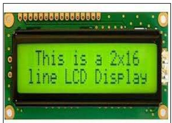
Fig -2: LCD Display (2 x 16)
