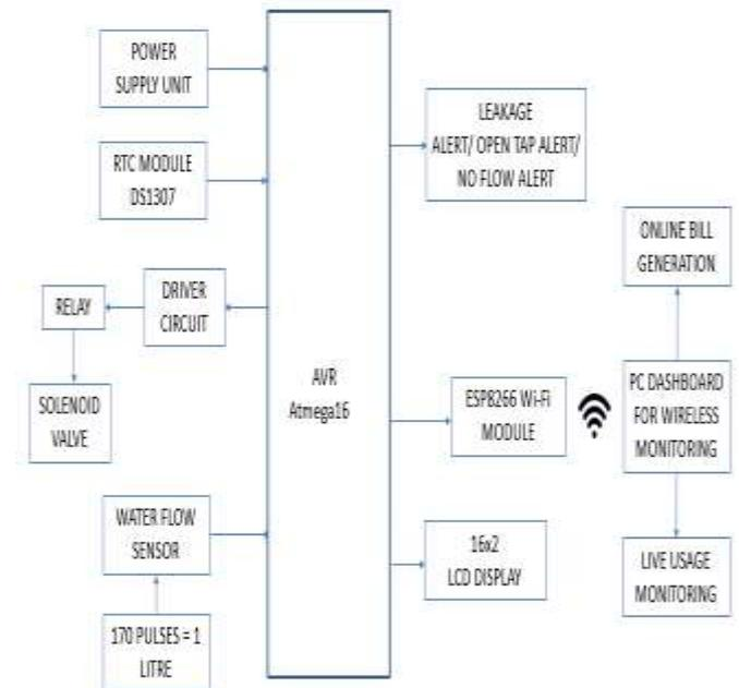
Fig -1: Block Diagram for the Digital Water Management and Automatic Billing System
