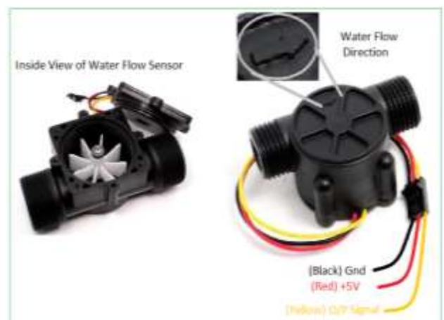
Fig -3: Water Flow Sensor
