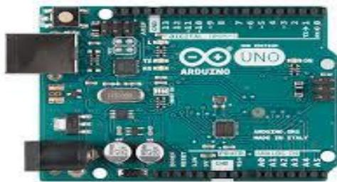
Fig-3: Arduino UNO Microcontroller
