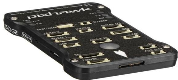
Fig-5: Pixhawk Flight Controller
