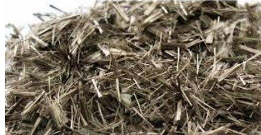
**Fig -1: Basalt Fibre**
