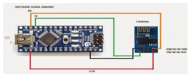
Fig -7: Interfacing of WI-FI module with Arduino
