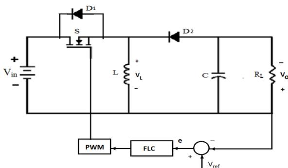
Fig -2: Buck-boost DC/DC converter system
