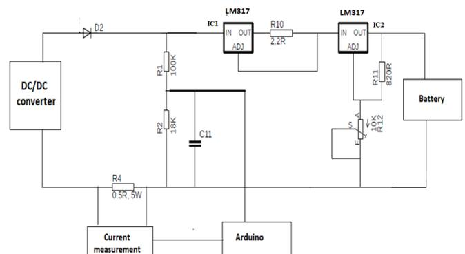
Fig -3: charge controller circuit diagram for battery
