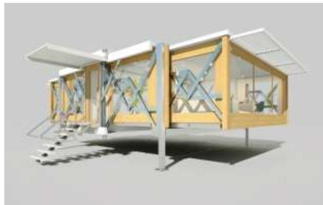
**Fig 14:- Deployable Folded Portable Structure manufactured by tenfold engineering based on scissor mechanism.**
