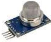
The gas sensor used is MQ6. This is an LPG gas sensor. It is used in detecting the gas leakage in consumer and in industry levels. The sensor requires a supply voltage of 5V. The sensor is used to detect gases like LPG, iso-butane, propane. The sensor is highly sensitive. A potentiometer is used to adjust the sensitivity of the sensor.
