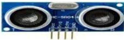
Ultrasonic sensors use the ultrasonic waves to measure the distance. The distance is calculated based on the transmitted and received signals. The distance is calculated with the formula  $L=1/2 * T * C$ .
