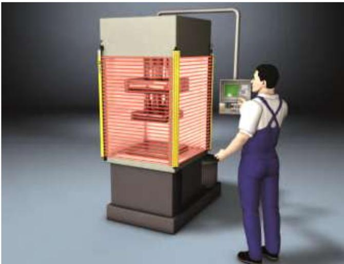
Fig -6: Model of Safety Light Curtains
