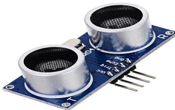
Determine distance to an object. One membrane produces sound and the other catches and reflects echo. The sensor detects the fuel level by the reflection of the echo. Non- contact distance measurements within a 10cm range. It can be varied according to the height of the tank.
