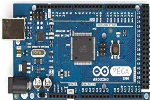
Arduino is an open-source electronics platform depends on easy-to-use hardware and software. Arduino boards are able to read inputs-light on a sensor, Twitter message or a finger on a button and turn it into an output-activating a motor, turning on an LED, publishing something online. The Arduino mega 2560 board is connected with the Ultrasonic sensor and LCD display.
