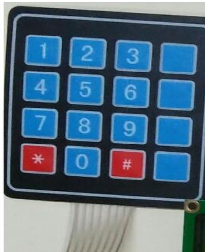
Keypad is used to enter the mileage of the vehicle. Enter and reset buttons are processed through the keypad. It is then connected with the Arduino mega 2560 board. The mileage can be reset for different values of different vehicles.
