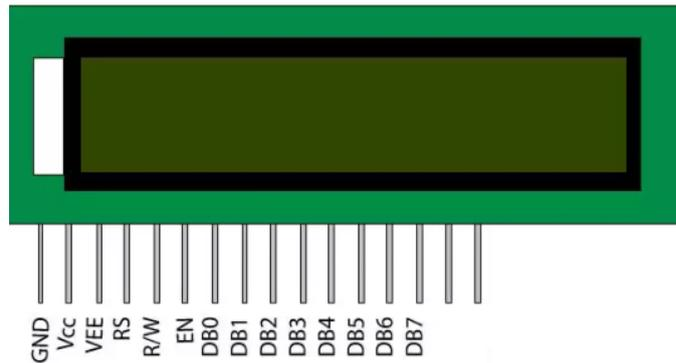
LCD (Liquid Crystal Display) screen is a display module of an electronic device and has a wide range of applications. A 16 x 2 LCD display can be used to display 16 characters per line and there are 2 such lines. It is used to enter the mileage and to display the actual distance to be traveled by the vehicle driver.
