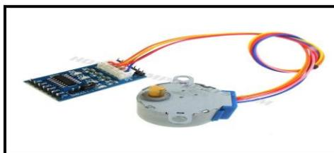
Fig -2: Stepper Motor with Drive
