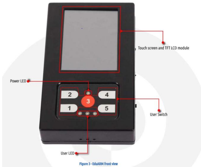
Figure -1: EduARM Development Board
