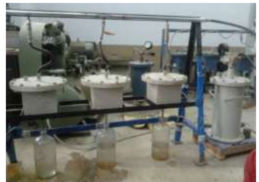
Fig-6: Permeability Testing Arrangement
