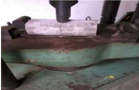
Fig -5: Split Tensile Strength Testing Arrangement
