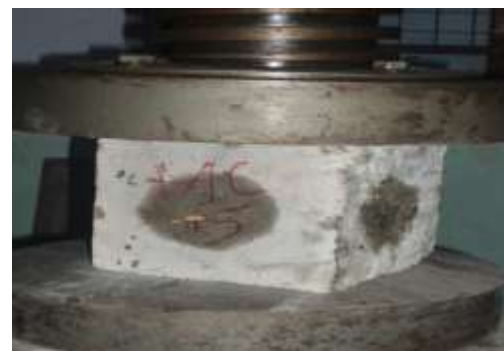
Fig -4: Compressive Strength Testing Arrangement
