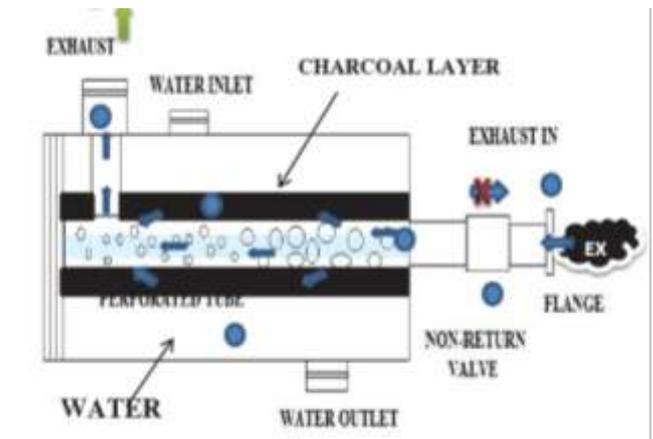
The exhaust gases passed into the emission controller, the perforated tube converts high mass gas bubbles into low mass gas bubbles after that they come into contact with lime water they chemically react with lime water and pass through the charcoal layer which again purify the gases. Its porosity remains constant in water. Since the charcoal layer is covered with metallic mesh which is filled with the lime water.
