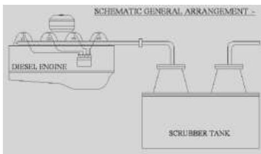
A small opening is at the top of the container to pass the exhaust gases in atmosphere and a drain plug is provided at the bottom of the container for periodically cleaning of container.
