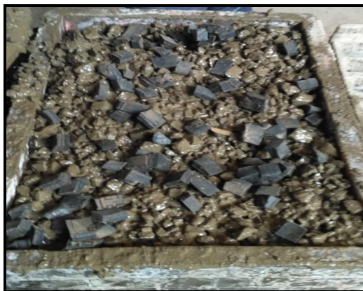
Fig -2: Presence of rubber chips in paver blocks.
