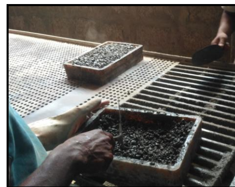
Fig -4: Placing of blocks on vibrating platform.
