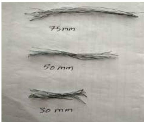
Figure 1: Steel fiber of crimped shape with different length
