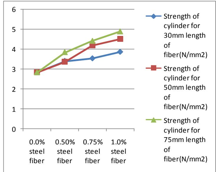
Chart 4: Split tensile strength of cylinder for 28 days
