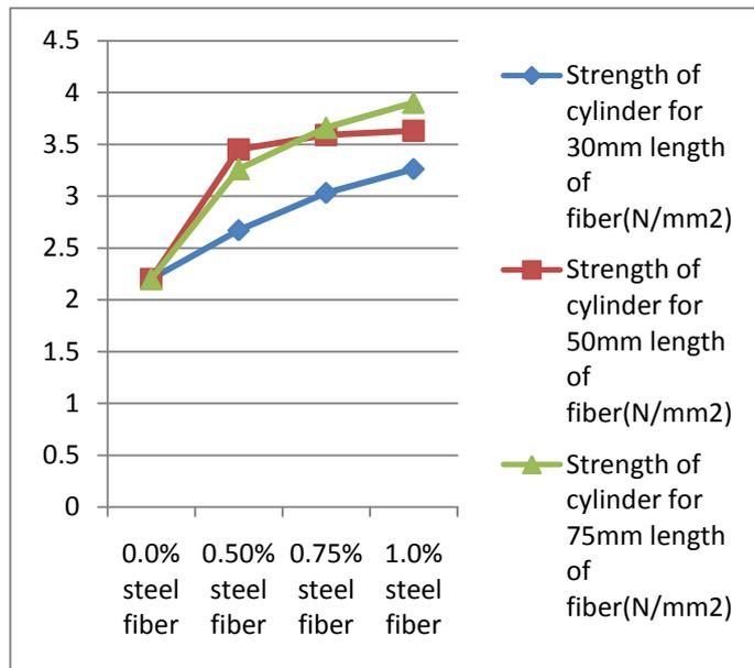
Chart 3: Split tensile strength of cylinder for 7 days
