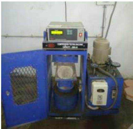
Figure 3: Compression testing machine testing of cylinder
