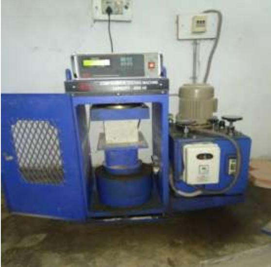
Figure 2: Compression testing machine testing cube
