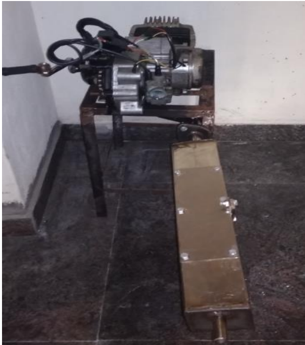
Fig-9: Experimental setup of zeolite silencer
