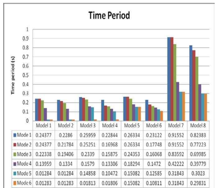
**Fig - 4** Time period for the building on plane and slope ground
