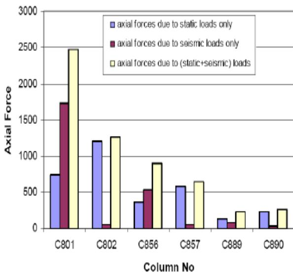
Fig -1 Column Axial Forces of the Studied Frame
