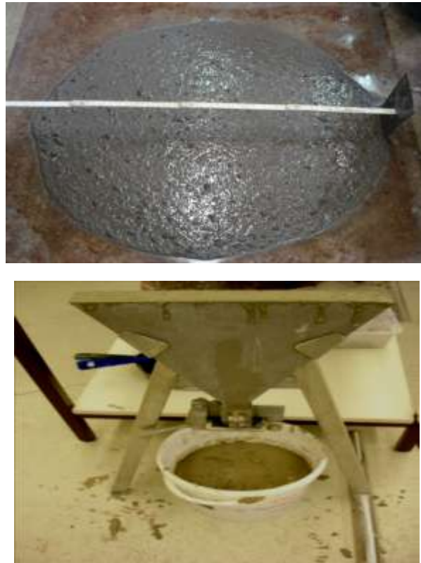
Figure 2.0: Fresh properties determination at concrete laboratory
