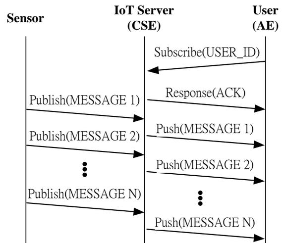
Fig – 2: The Active scheme of D<sup>2</sup>ATC mechanism.
