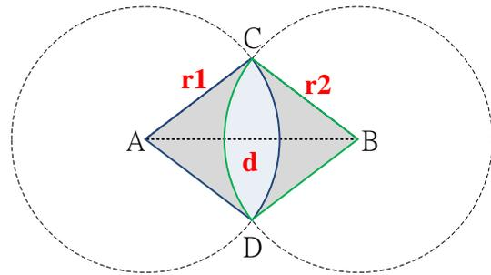
Fig - 4: The communication overlapping situation between two sensors A and B.
