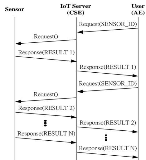
Fig – 3: The Passive scheme of D<sup>2</sup>ATC mechanism.
