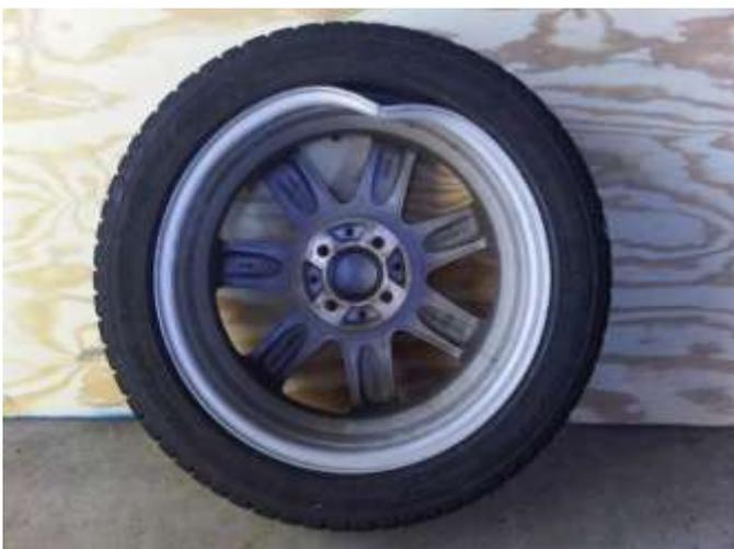
**Fig -3: Bent rim of a car provided by "Rim Blades USA"**
