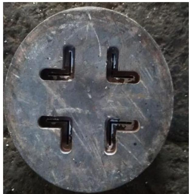
Fig 4: multi cavity extrusion die
