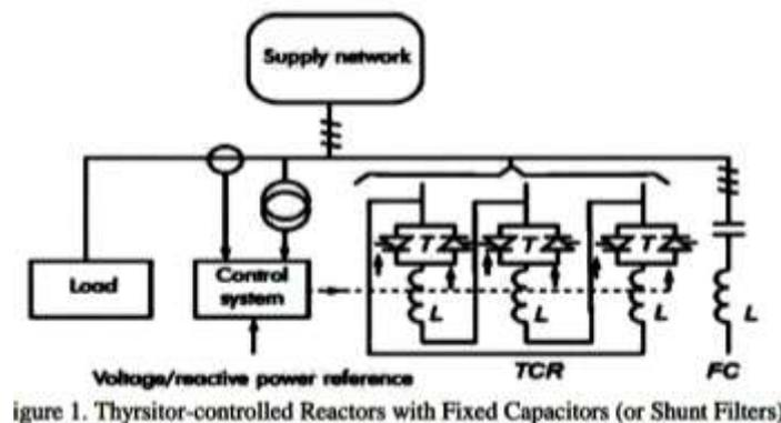
**Figure 1.** Thyristor-controlled Reactors with Fixed Capacitors (or Shunt Filters)
