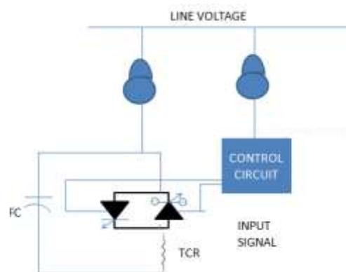
**Fig: 2.1** SVC Shunt with Transmission Line
