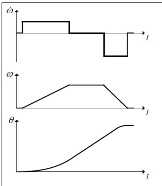
Fig - 8: Acceleration, Speed and Position.
