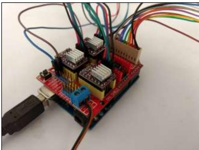
Fig - 10: Electronic Circuit of SCARA robot
