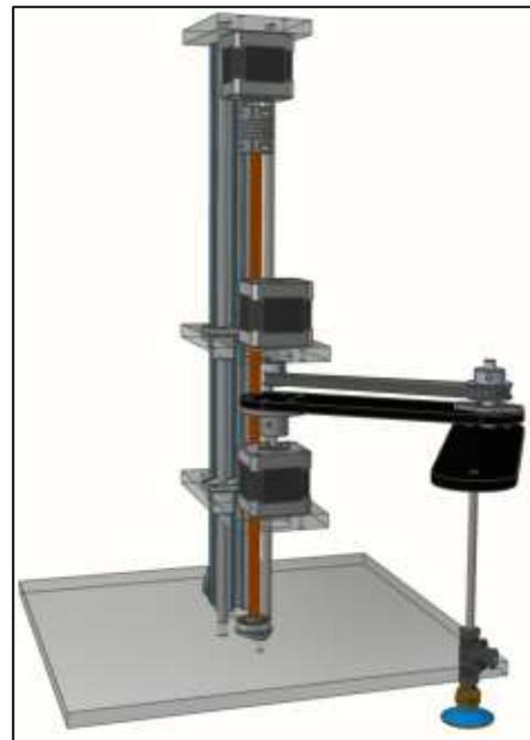
**Fig - 3:** 3D Model of Robotic arm.
