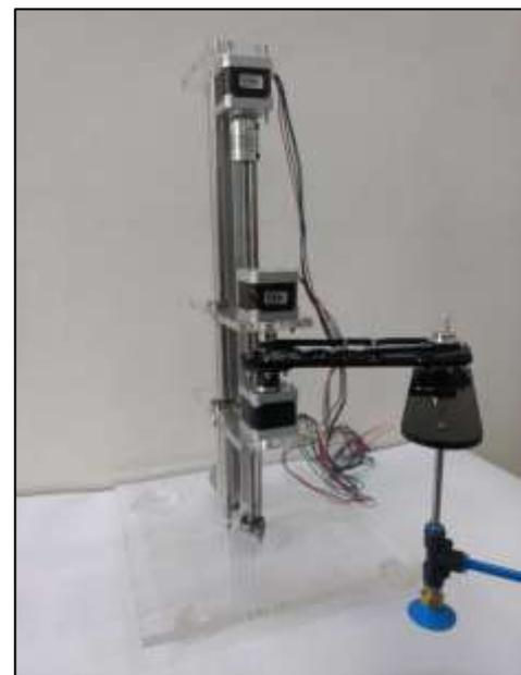
**Fig - 4:** Actual model of Robotic arm.
