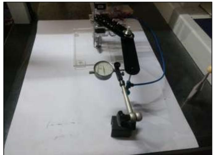
Fig - 12: Setup for repeatability trials
