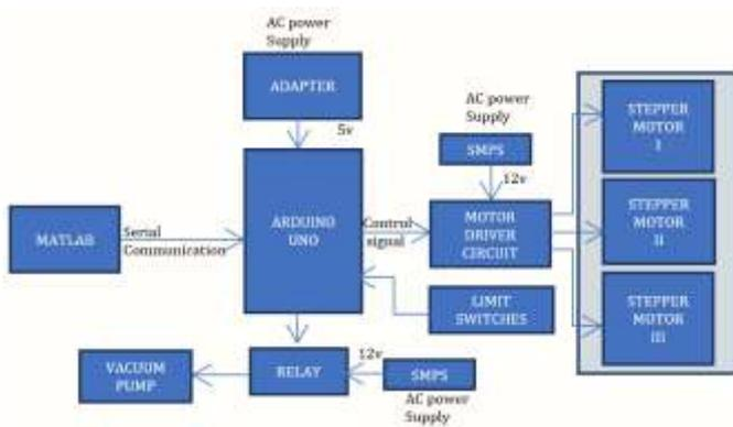
Fig - 9: Block diagram of SCARA robot
