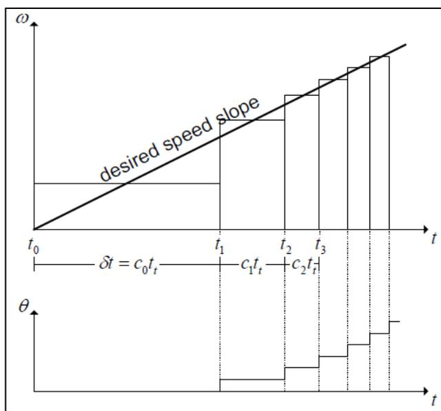
Fig - 9: Speed profile against stepper pulses
