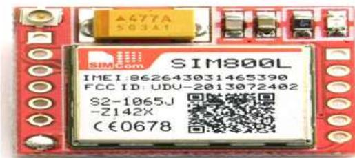
Fig 5: SIM800L GSM / GRPS module
