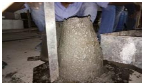
Figure 1: Slump Cone Test
