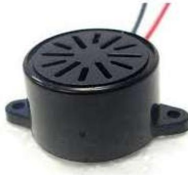
It is a device which is used to produce sound in case of an emergency. It consists of a small electromagnetic circuit consisting of a coil and a magnetic disk. When a current is passed through the coil, the coil produces fluctuating magnetic field due to which the disk vibrates at a frequency equal to that of an input drive signal.
