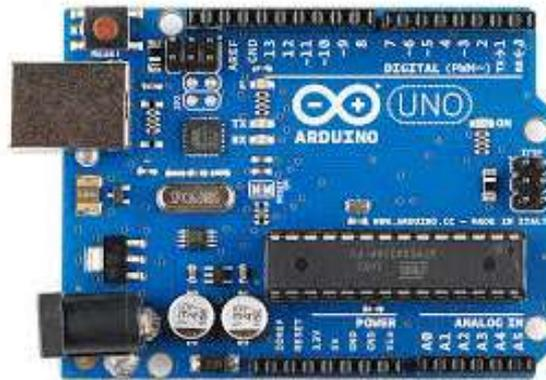
The Atmega 328 is a low-power CMOS 8-bit microcontroller which is based on a RISC architecture. It is powerful enough to execute instructions in a single clock cycle. It achieves the throughputs approaching 1MPS per MHZ allowing the system designed to optimize power consumption versus processing speed. Power saving is one of the important characteristics of it.
