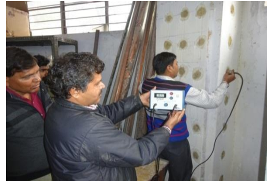
Fig: 2 UPV Test by Direct Method on Column
