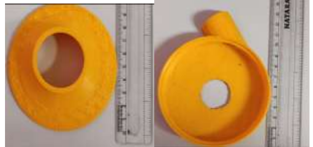
Fig-8: 3D Printed Volute Casing
