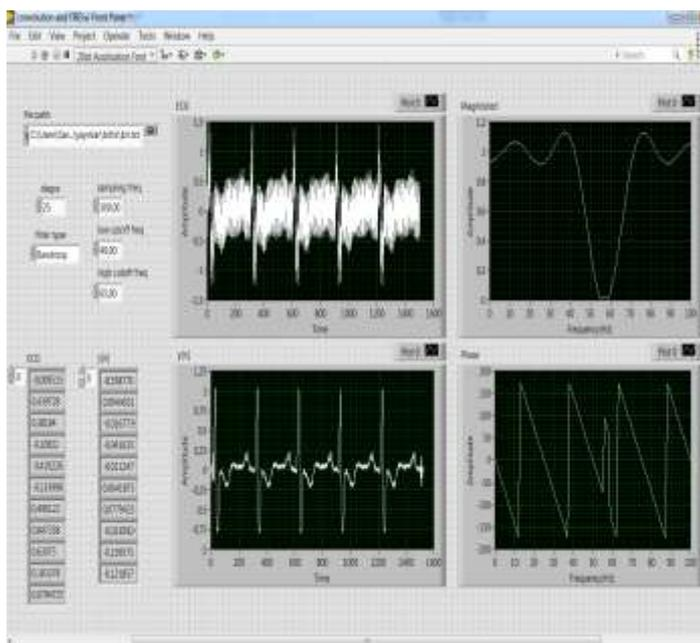
Figure 4. FIR Filter Front Panel
