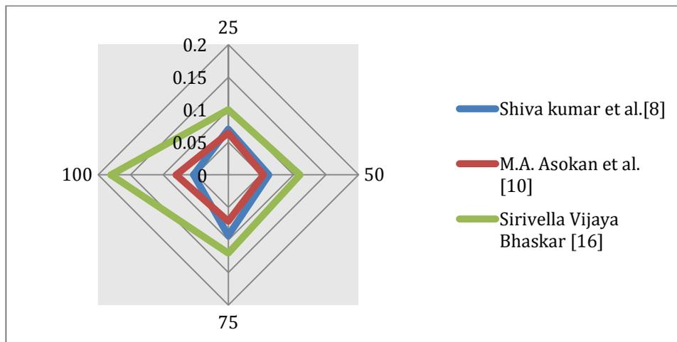
Fig.7:- Co emission for B20 in % Volume vs. load
