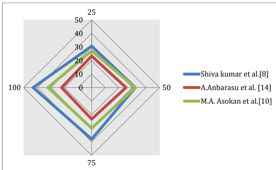
Fig.3:- NO<sub>x</sub> emission for B20 in PPM vs load
