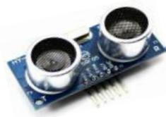
**Fig -2:** Ultrasonic sensors
