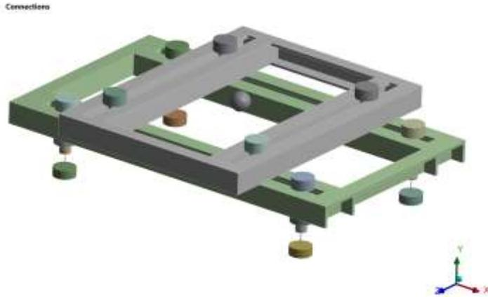
Fig-7 Isolators at four fixation locations
