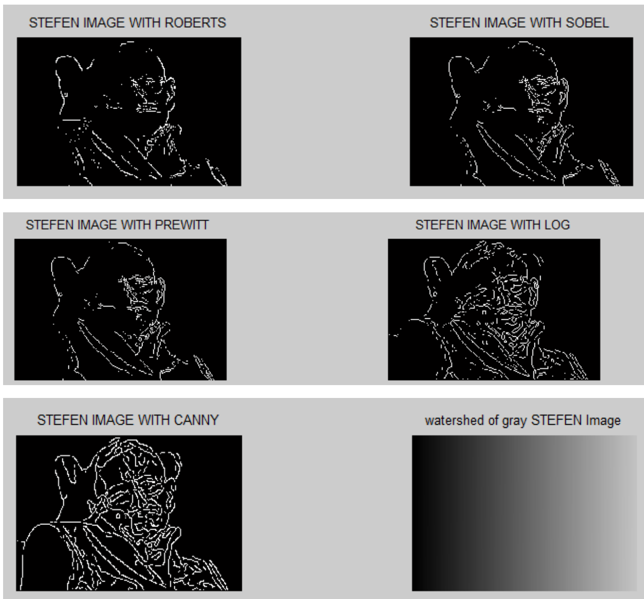
Fig: 4.1.1 result image with various operators
