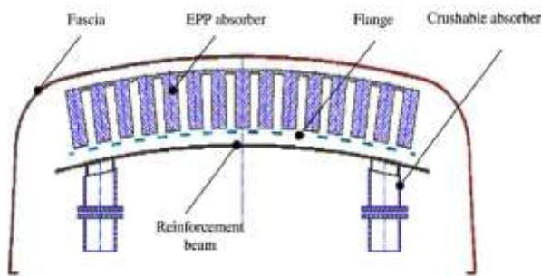
Figure 8: Cross section of Front Area in bumper system
