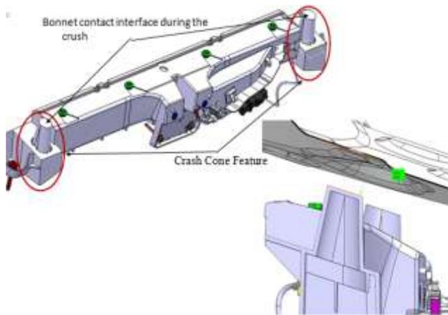
Figure 14: Crush Cone Feature in part
