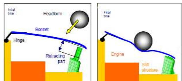
Figure 12: Crush Cone Feature Concept
