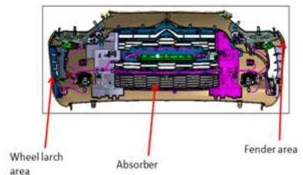
Figure 5: Typical Front bumper system, Rear view
