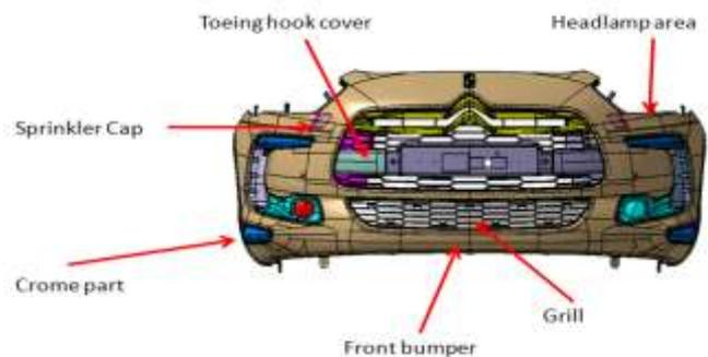
Figure 4: Typical Front bumper system, front view
